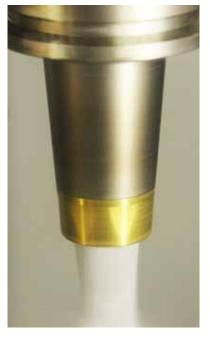
**COOLCAP®** in action: uniform, ring-shaped cooling jet
