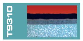
Fine grained functional gradient substrate
